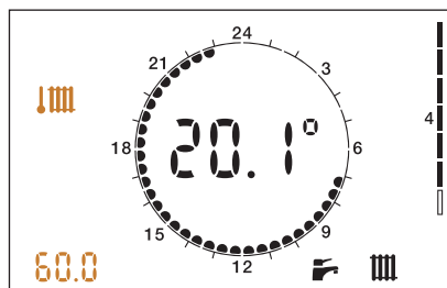
Heating flow temperature
