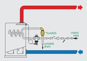
\* The discharge from a temperature relief valve should be through a tundish to a suitable drain.
