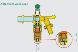
When the temperature of the water in the supply pipe drops below 3°C, the obturator of the antifreeze device opens and drains off the water. The obturator closes when the medium temperature returns to 4°C.
