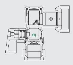
The DN15 valve complies with the minimum flow way for reduced bore valves in BS EN 13547.
