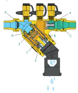
The check valves (3 and 4) close as the pressure upstream (A) drops.
