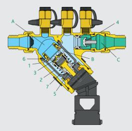
Under normal flow conditions, both check valves (3 and 4) are open, while the pressure in the intermediate chamber (B) is always lower than the inlet pressure (upstream A) by at least 14 kPa due to the pressure loss caused by check valve (3).
