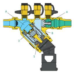
The check valves (3) and (4) are now closed. Since the pressure in the upstream zone (A) is still at least 14 kPa higher than the pressure in the intermediate chamber (B), the discharge valve (5) remains closed.
