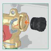
The special connection system does not allow installation errors. The fixing clip only fits into the corresponding groove if the element to be connected is in the correct position.
