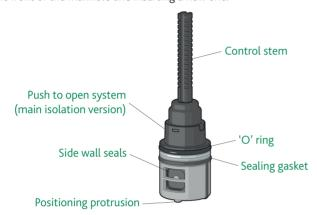
There are two types of cartridge, one used in manifolds with individual isolation valves and one designed for versions with main isolation valves
