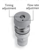
It is possible to progressively vary the timing and flow rate without removing the cartridge from the tap body using a 2mm hexagonal wrench.
