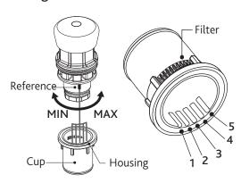
The flow rate depends on the position of the reference (located on the cartridge body) in the seat of the plastic cup.
